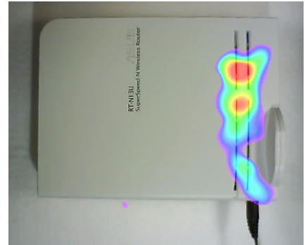
Figure 1: Acoustic image showing broadband noise from a router
