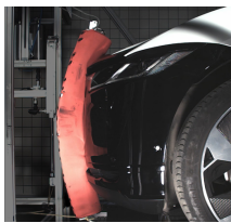
Image 1 ((Test with aPLI legform impactor, measX_leg-test_srcEuroNCAP.jpg ))
